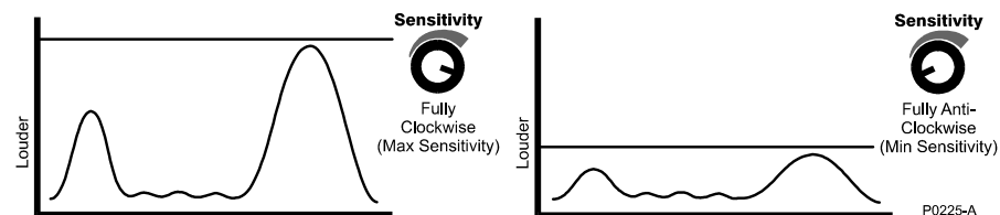
Figure 15 – Sensitivity Control (The audio output is amplified according to the Sensitivity setting)
